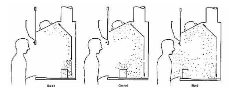
Move work at least six inches inside the face of the fume hood. This minimizes the effect of crossdrafts and eddies created by the hood operator or by occupants walking by the hood. Also, keeping windows and doors closed will control cross-drafts.
