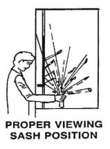
**Work with the hood sash partially or completely closed.** If this is not possible, additional Personal Protective Equipment (PPE) should be used to ensure adequate protection.
